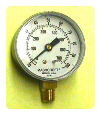
The meter illustrated above is the standard meter used most commonly in molasses applications. Pressure indication is 0-100 PSI.
