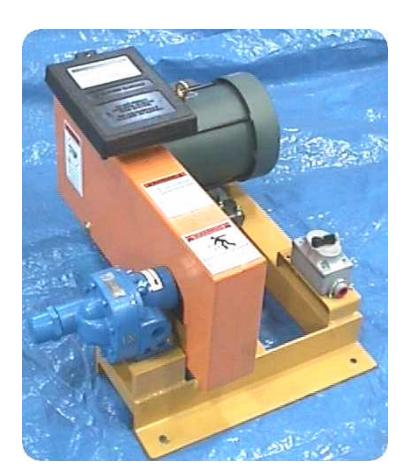
3 HP molasses/fat pump with adjustable built in by-pass valve. Complete with motor and drive. 200 pounds
