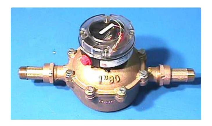
The Model SC-ER-H Molasses Disc 1" Meter with Bronze chamber, shown above, measures the flow of molasses or other liquids through a pipe. The illustrated #PFT2E Electronic Transmitter mounted on the meter. transmits flow information to the Model PC100 Panel Mount Industrial Process Controller shown at right. The controller can display and process the liquid flow information in any unit of measurement. The meter/transmitter weighs 11 pounds. The Controller weighs 2 pounds
