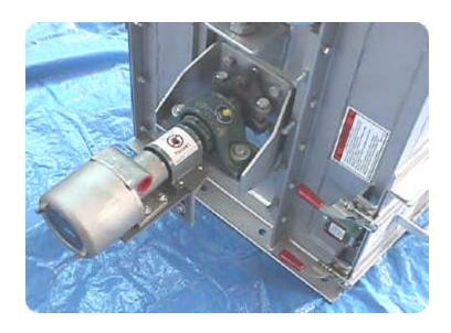
Boot details illustrate high temperature roller bearings, fixed and floating mounted outboard from boot housing. Shaft seal is a gland compression arrangement using KEVLAR packing rated at 500 degrees F.
