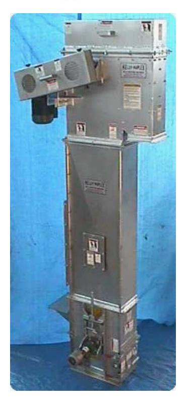
Bucket Elevator with 1-1/2 HP drive operating at 206 FPM with C188 combination chain and 6" x 4" Style AA malleable iron buckets. Note the quick opening maintenance panel in the boot and the Model CMS motion switch mounted on the boot shaft.
