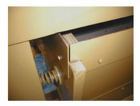
The carefully constructed wooden grader shoe is suspended to the integrated machine steel frame with isolation springs in four places, as illustrated above. The single motor drive, which operates all functions of the Kelly Duplex Corn Cutter and Grader. illustrated in the photo to the right. Overall operation is very simple with minimum maintenance
