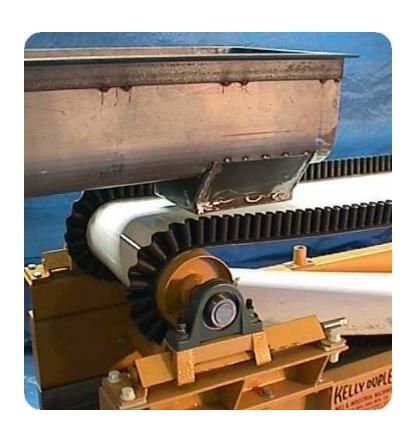
Screw feeder delivers material to the ConveyAccord Belt Conveyor at a uniform and momentarily controlled rate.
