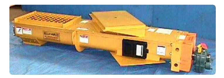
Twin spiral counterrotating 6" screw feeder receives material from upstream and provides a relatively uniform flow rate to processing machinery downstream. In this case material is fed to an 18" Kelly Duplex ConveyAccord belt conveyor (69141-H13054). This feeder unit is equipped with a variable speed hydraulic drive, a panel for viewing flow rates covered with a 2" x 2 receive material from upstream, an end discharge, and a pass through discharge.
