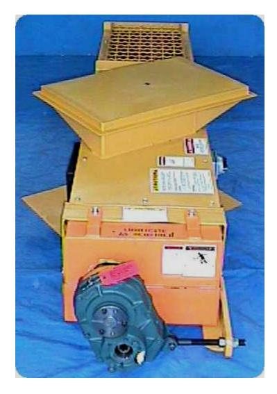
View from discharge end. Twin 6" spirals and viewing grate are shown View from drive end. Shaft mounted gear reducer with plug-in hydraulic motor mount, tie rod and tie rod anchor are shown.
