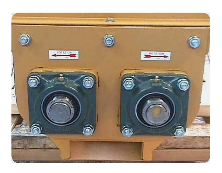
View shows discharge end of screw feeder where material exits the feeder and is placed onto a belt feeder.
