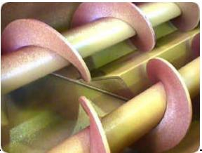
Twin, counterrotating spirals are shown in these views. The by-pass discharge can be seen in the view above.
