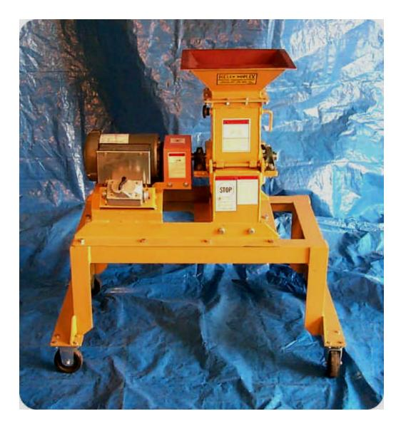
The Kelly Duplex Model LM6 Hammermill features a 6" wide x 10-1/2" diameter rotor. The mill weighs about 150 pounds and is a compact 24" high including a 12" x 12" inlet hopper. Hammer tip speed at 1750 RPM is 1530 FPM. Hammer tip speed at 3550 RPM is 3100 FPM. Power input can range from 1 to 5 HP depending on intended application.
