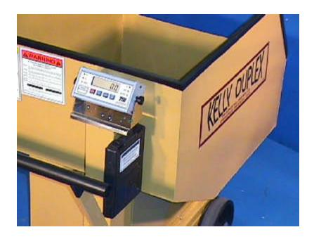
View of battery operated digital indicator. Indicator provides readout up to scale capacity of 1,000 pounds graduated either in pounds or kilograms
