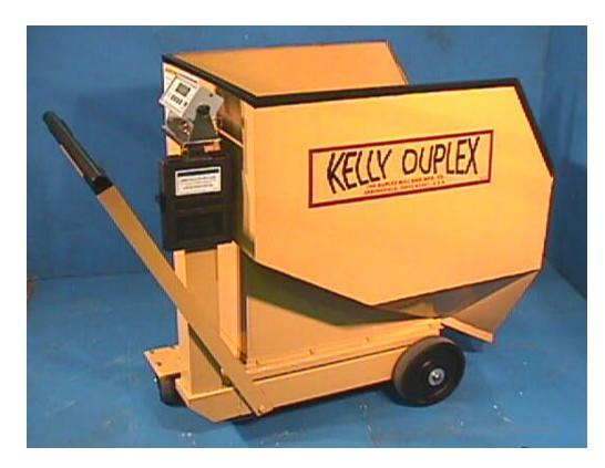
View shows large front wheels and rear swivel caster with brake. Floor level discharge with easily operated slide gate delivers weighed materials out the front bottom of the bulk body.
