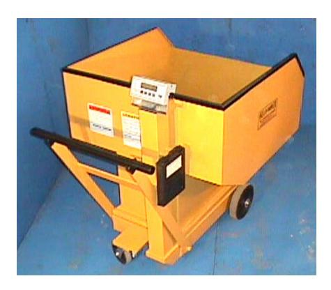
Views illustrate the 25 cubic foot bulk body, 1000 pound capacity scale with battery operated digital indicator, attached operators manual case, 10" molded-on rubber wheels, rear swivel caster with brake in rear, heavy duty pushbar, and convenient discharge slide control. The digital weight indicator provides readout up to scale capacity of 1,000 pounds graduated either in pounds or kilograms
