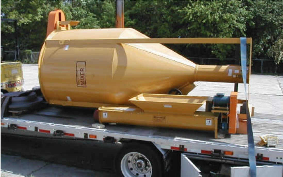
Transportation of a vertical mixer is usually accomplished economically through the use of a contract carrier. In these views the vertical mixer and screw feeder are shown loaded on a flat bed truck and tarped for transportation.
