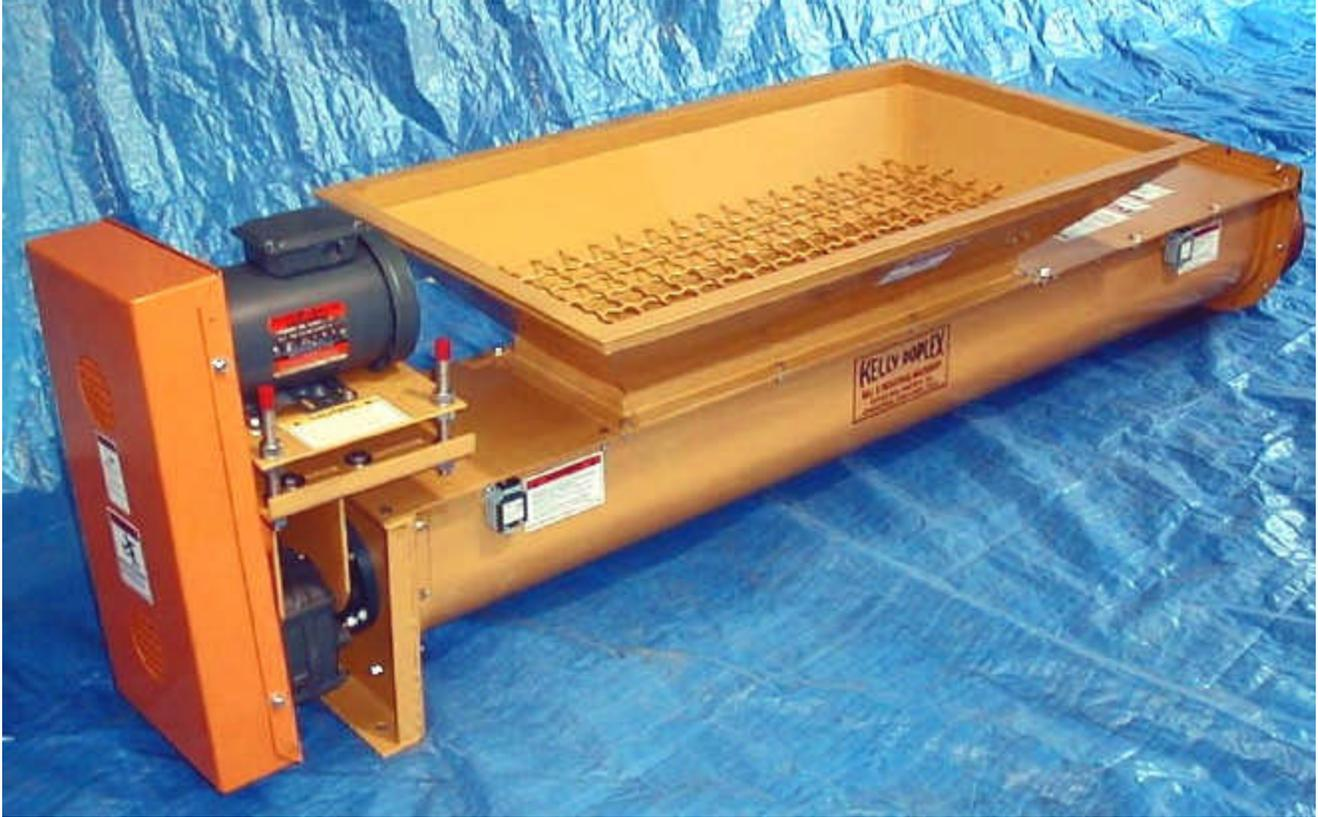
The vertical mixer spiral is force fed with a 9" screw feeder directly connected to the mixer downtube 6" above floor level. The 24" x 48" x 45 degree inlet hopper provides for convenient and metered loading of the mixer batch. The top of the hopper is located just 28" above floor level
