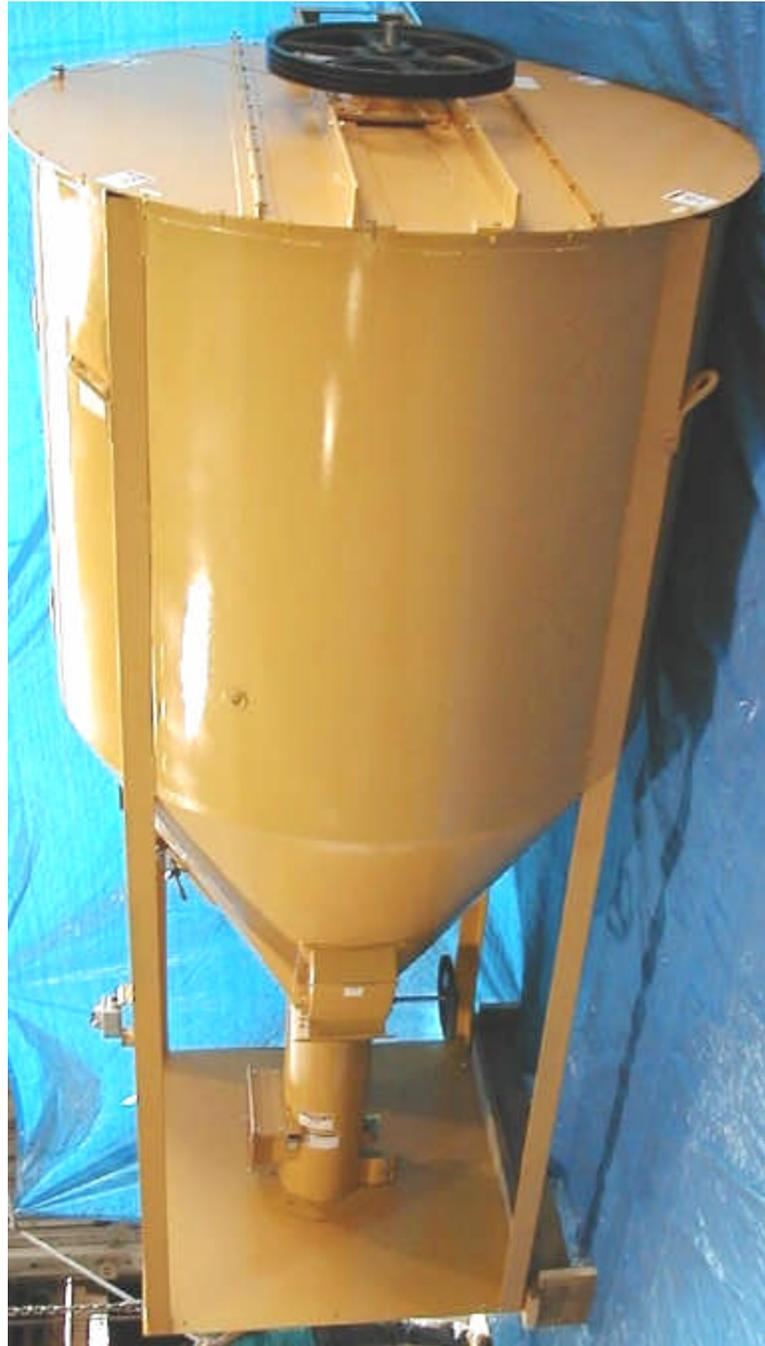
Overall view of vertical mixer illustrates 10" rack and pinion discharge gate and force feed inlet in down tube just 6" above the floorplate. V-belt drive is shown at the top.
