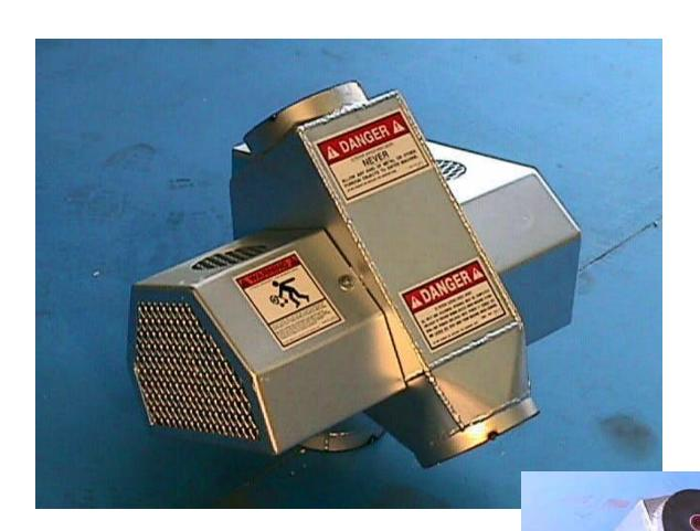
Views here illustrate the protective covers mounted over the air cylinder valve actuation assembly, the position limit switches and the solenoid air valve.
