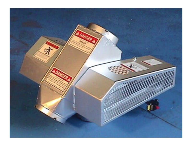
This 6" x 2-way diverter valve is air cylinder operated and features a 45-degree material flow. The tolerance of high temperatures is enhanced by the use of TEFLON shaft seals, high temperature bearings, VITON sealed air cylinder and stand-off mounting of position limit switches and solenoid air valves. Constructed of carbon steel the entire fabrication is painted with high temperature aluminum paint.
